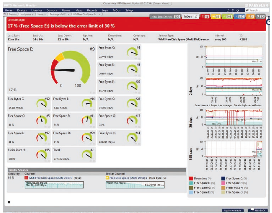
The wide, colored status bar in PRTG shows the administrator clearly whether the monitored resource is alright or not.
